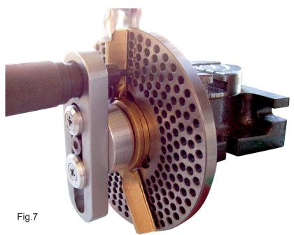
Loosen slightly the locking screw on the quadrant arms, and spread the right-hand one till the inner, bevelled edge is adjacent to the 28th hole on row 49. Now lock it so that it can't move. Now your all set to go!
